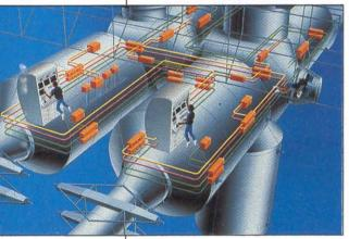
Computers will play a key role in the daily operations of the space station. Because science is the primary mission, NASA is designing a computer system to manipulate millions of megabytes of data gathered from up to 30,000 sensors aboard Freedom.
